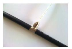
3. Feed over additive shunt into the PA hose (6 mm) after the LPG jet (inline):
