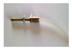
2. Feed over additive shunt into the rubber hose (NW 5-6) after the LPG jet:
