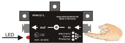
**Step 1:** Start the vehicle and activate gas operation. The dosing module is now provided with power and remains in Set-up ready mode (LED lights up yellow) for 30 seconds.
