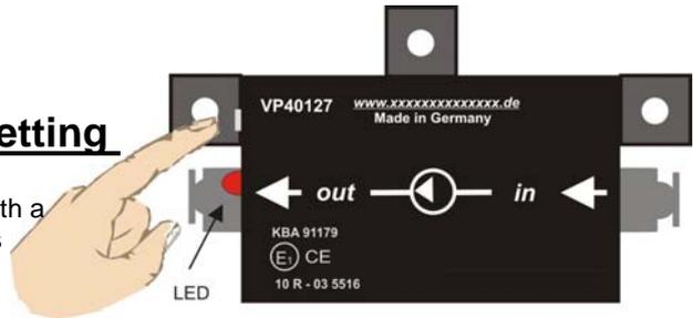
**Step 1:** Start the vehicle and activate gas operation. The dosing module is now provided with power and remains in Set-up ready mode (LED lights up yellow) for 30 seconds.
